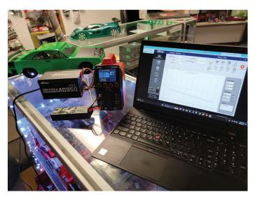
in-depth analysis of a battery pack, like the SMC unit we tested. Even without the PC connection, we could use the RDX2 to see battery information, including the internal resistance (IR), which is essential in selecting the best battery packs for high-performance applications. The charger also has the ability to use its power supply to turn a charging port into a DC output to power a tire warmer.
