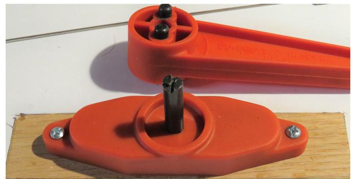
I first tried the thinner wire and the "Z" bend side. This is the bend I use most often. For the 1-meter wingspan models, I will make a bunch of rods with the "Z" bend and a 3 to 4 in. length of straight wire. They are then bound to carbon rods or dowels later for complete pushrods. I have spent many hours with Ed Bojan at NRHSA, watching him effortlessly crank out "Z" bends. Yes, it is that easy with this tool.
